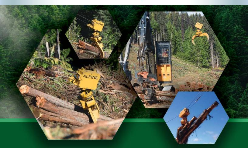
Grapple pivots from carriage for smooth 360 degrees rotation Grapple-mounted wireless camera system
