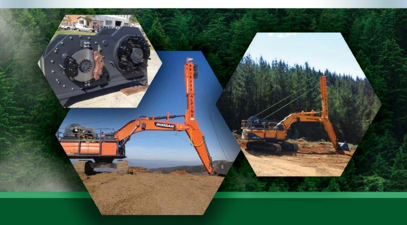
DOUBLE DRUM ALPINE SHOVEL YARDER CONVERSION KIT, THAT TRANSFORMS YOUR EXCAVATOR INTO A POWERFUL DOUBLE DRUM, UPHILL "LIVE SKYLINE" GUY-LESS GRAPPLE YARDER. THE POWERFUL SKYLINE DRUM IS ALSO EQUIPPED WITH LEGAL SKYLINE SLIPPING BRAKES, THAT ENABLES THE YARDER TO OPERATE AS A "STANDING SKYLINE" SYSTEM, USING CONVENTIONAL MULTI-SPAN SKYLINE CHOKER CARRIAGES.
